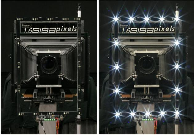
**Figure 1: Gigapixel 3D camera.** We equipped Microsoft Research Asia’s 1.6 gigapixel camera with 16 LEDs to realize nearby light photometric stereo.
