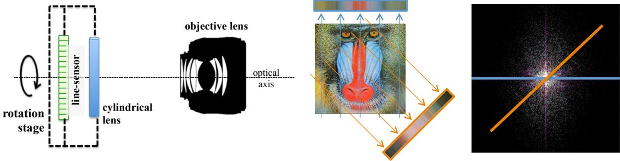
(a) Optical setup of the proposed light-modulator-free design for compressive imaging (b) Imaging model and its representation in Fourier domain
