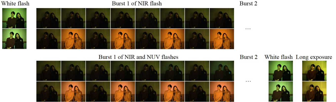
Fig. 5. An example scene from our dataset. We show a series of image pairs where the upper image is from cam_1 (RGB) and the lower image is from cam_2 (NIR-G-NUV). Burst 2 is omitted for space, as it resembles burst 1. The flash images with different exposure time use different analog gains such that they have same level of brightness. These linear images have not been white balanced, hence their green or orange appearance.
