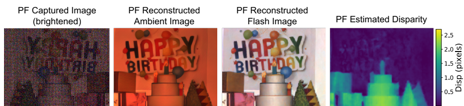
Fig. 3. Single-shot flash/no-flash imaging with patterned flashlight. When ambient and flash illumination have very different spectrum, our method can be used to jointly reconstruct ambient and flash image, and the scene disparity.
