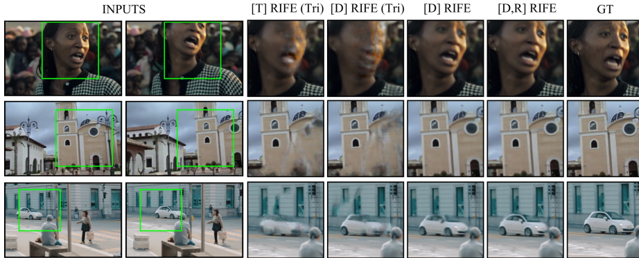
Fig. 1: Additional comparison of qualitative results. [T] RIFE (Tri) denotes RIFE [1] trained in a fixed time indexing paradigm (Vimeo90K triplet dataset [8]). [D] RIFE (Tri) denotes the model trained using distance indexing. All models use uniform maps.
